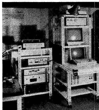
Fig.1. An experimental radiometer system consisting of a three-band radiometer (left) and a microcomputer (right).
